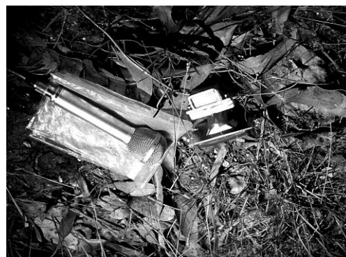
Figure 7. Field playback setup with microphone (Beyer M 88) and loudspeaker (Kaltro HTM-2 tweeter) directed at a calling male of the Victorian Smooth Froglet which is concealed in the patch of grass in the lower right of the image.
