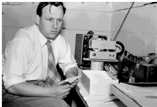
Figure 4. The author with Philips GM 3156 cathode ray oscilloscope and attached Southern Instruments M 726 continuously recording 35 mm camera with M 729 motor unit. Also shown is a Pyrox Magictape TR-ST1 tape recorder for playback and A. J. Williams SR4 resonant reed frequency meter to indicate the AC mains frequency as a check for calibration of the film speed. Photograph taken ca 1954.
